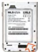
In order to remove the battery from the device, pull it up by placing your finger in the appropriate niche, as shown in the picture to the left.
